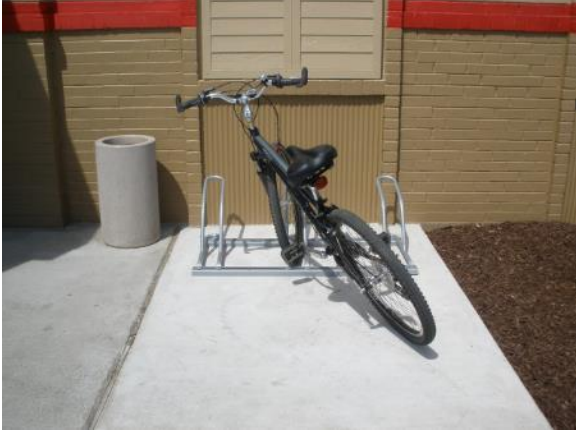
Figure 3. Another style of “wheel bender” bicycle rack. Source: Reimagine Round Lake Beach ( https://reimagine.rb.com/2014/06/02/about-hardees-bike-rack/ ).
