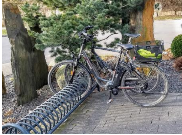
Figure 4. Another style of “wheel bender” bicycle rack. Source: Madison Bikes ( https://www.madisonbikes.org/dispatch_from_germany ).
